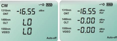
If you want to change current optical power as reference value, please hold (>2s) REF button in the measuring mode, meter will finish this job after one "beep", value on the display is result from the comparison with the reference value (unit is dB).
