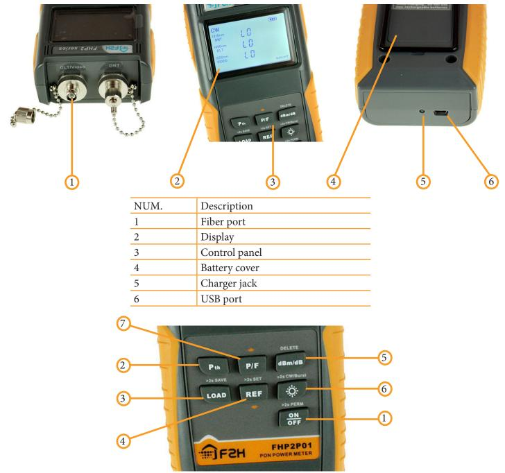
Buttons of this meter have secondary function, normal push to use the function which indicated on the button, hold (>2s) to use the function on the panel, all the functions have been listed as follow:
