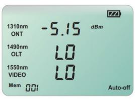
Item "Mem 001" at left bottom means the first group of data, it stand for the sequence of saved data, the value above is the power value for relevant wavelength.
