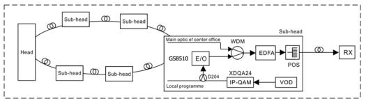
Applied in second transmission of sub-station (FTTx), supply with IP/QAM, VOD VAS
