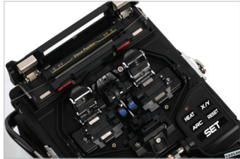
3) Moving the fibers and heat-shrink tube to the heat oven
