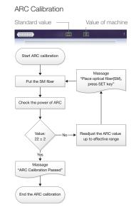
Important: 1) Always use SM fiber only 2) To keep in best splice condition, following the procedure.
