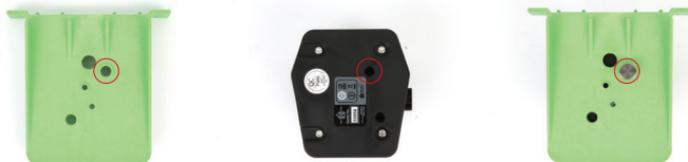
Fix the cleaver on the cleaving table by matching screw.
