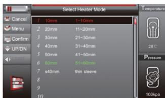
③ Press “Up” and “Down” to select the heater mode, and press
