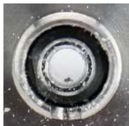
Top of the contaminated connecting bar
