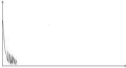
If the tested trace is just like the figure shows above, this might be caused by several reasons like: a bad connection between the connector and the launching port, the optical pulse cannot be launched into the optical fiber or a short distance broken point of the tested fiber from the initial connection and the preset testing distance and pulse width is larger.
