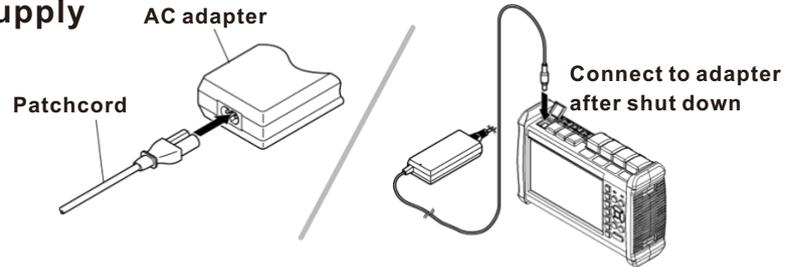
Once connect to AC adapter , power indicator turns red(if it is not fully charged), adapter is charging the battery , after fully charged power indicator turns green.
