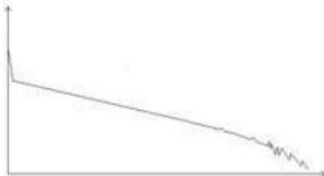
This situation often happened in a long distance testing, caused by under-range dynamic range of the OTDR that the energy of it can not support a long distance transmission or caused by a under-range preset testing range of distance or pulse width corresponding to the actual fiber length. To avoid this situation, adjust the testing distance and the pulse bigger and extend the sampling time.
