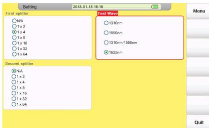
Set "First splitter", "Second splitter" or "Test wavelength" option according to the actual condition of your fiber under test. After setup is finished, press **[ESC]** back to test interface and press **[F1]** to start the FLM test.
