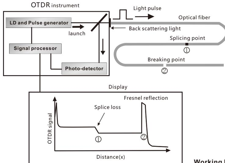
Working Principle of OTDR
