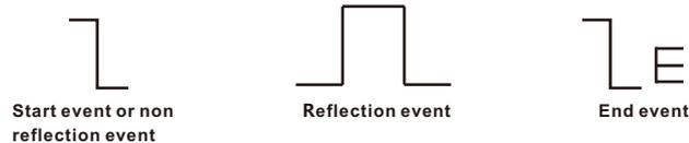
The events on trace are all the points that the value of power loss fluctuates abnormally. It usually contains various types of connection and bending, crack, broken and etc. The event points marked on trace with special marks are the abnormal points in a fiber that cause the excursion of a normal trace.
