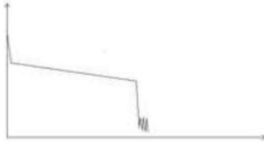
The situation that there is no reflection peak at the end of a trace shows above should be paid attention on. If the distance of the tested fiber is available and the distance shown on OTDR is not equal to the original distance, this shows that the fiber might be broken down or twisted and the bending radius of it is over limited. The distance shown on OTDR is the position of the fault point.
