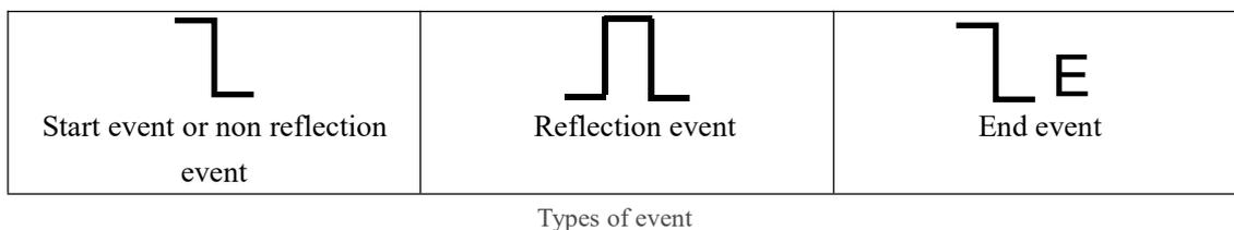
The events on trace are all the points that the value of power loss fluctuates abnormally. It usually contains various types of connection and bending, crack, broken and etc. The event points marked on trace with special marks are the abnormal points in a fiber that cause the excursion of a normal trace.
