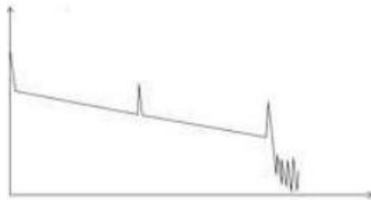
If there is additional reflection peak in a tested trace, this may be caused by a connection point or some other reasons. Anyway, appearance of the reflection peak shows that the two connecting surfaces of the connection are smooth. The smoother the connection surfaces are, the higher the reflection peak is.
