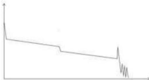
There is a common phenomenon that an obvious step is on the middle of a tested trace, it often caused by a fiber bending, fiber knot, being pressed by something heavy or a fuse splicing point. The step means a bigger loss of a fiber, it is also called event point. If the direction of it is downward, it could be called non-reflection event. If the direction is upward, we can call it reflection event.
