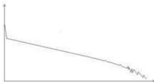
This situation often happened in a long distance testing, caused by under-range dynamic range of the OTDR that the energy of it can not support a long distance transmission or caused by a under-range preset testing range of distance or pulse width corresponding to the actual fiber length.
