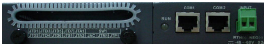
Figure 5-2 Front panel of the ESCM EMU
