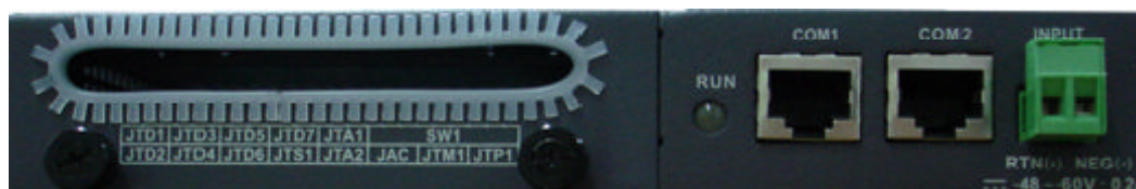
Figure 6-3 Front panel of the ESCM EMU
