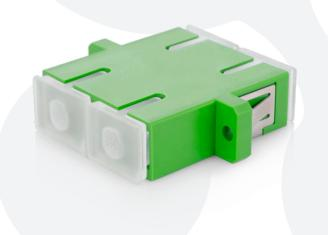
Adapter ConnLink SC/APC, SM, DUPLEX is a high quality double fiber optic adapter in green color from the renowned ConnLink brand. It is also available in GOLD class. The body of the adapter is made of a solid cast, which increases its durability, whereas a ceramic alignment sleeve guarantees the best transmission parameters. In addition, the adapter is equipped with a clip that allows it to snap into fiber optic enclosure ports without the need for screws.
