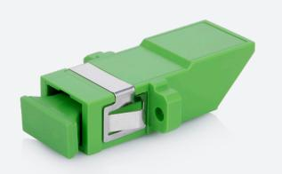
Adapter ConnLink SC/APC, SM, SIMPLEX, with FLAP is a high quality single fiber optic adapter (with flap for extra protection) in green color from the renowned ConnLink brand. The body of the adapter is made of a solid cast, which increases its durability, whereas a ceramic alignment sleeve guarantees the best transmission parameters. In addition, the adapter is equipped with a clip that allows it to snap into fiber optic enclosure ports without the need for screws.
