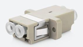
Adapter ConnLink LC/UPC, MM, DUPLEX (SC MOUNT) is a high quality double fiber optic adapter in beige (OM1/OM2), turquoise (OM3), pink (OM4), lime (OM5) color from the renowned ConnLink brand. The body of the adapter is made of a solid cast, which increases its durability, whereas a ceramic alignment sleeve guarantees the best transmission parameters. In addition, the adapter is equipped with a clip that allows it to snap into fiber optic enclosure ports without the need for screws.
