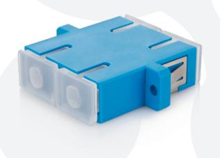
Adapter ConnLink SC/UPC, SM, DUPLEX is a high quality double fiber optic adapter in blue color from the renowned ConnLink brand. The body of the adapter is made of a solid cast, which increases its durability, whereas a ceramic alignment sleeve guarantees the best transmission parameters. In addition, the adapter is equipped with a clip that allows it to snap into fiber optic enclosure ports without the need for screws.
