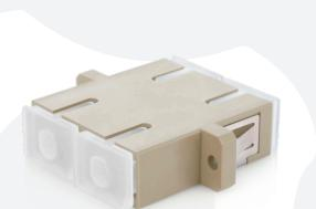
Adapter ConnLink SC/UPC, MM, DUPLEX is a high quality double fiber optic adapter in beige (OM1/OM2), turquoise (OM3), pink (OM4), lime (OM5) color from the renowned ConnLink brand. The body of the adapter is made of a solid cast, which increases its durability, whereas a ceramic alignment sleeve guarantees the best transmission parameters. In addition, the adapter is equipped with a clip that allows it to snap into fiber optic enclosure ports without the need for screws.
