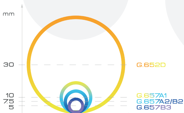
Minimal bending radius according to fibre type
