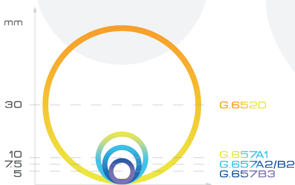
Minimal bending radius according to fibre type
