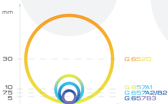
Minimal bending radius according to fibre type
