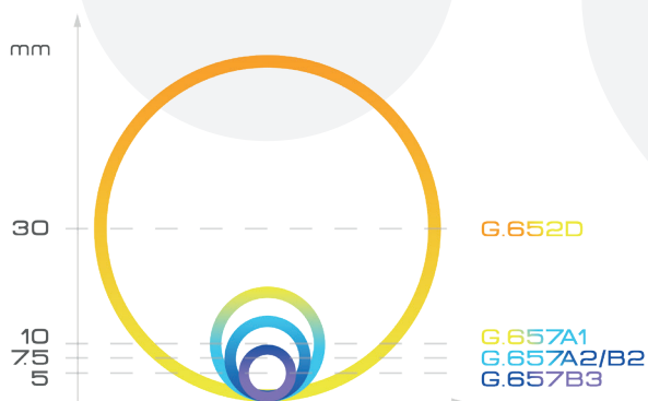
Minimal bending radius according to fibre type
