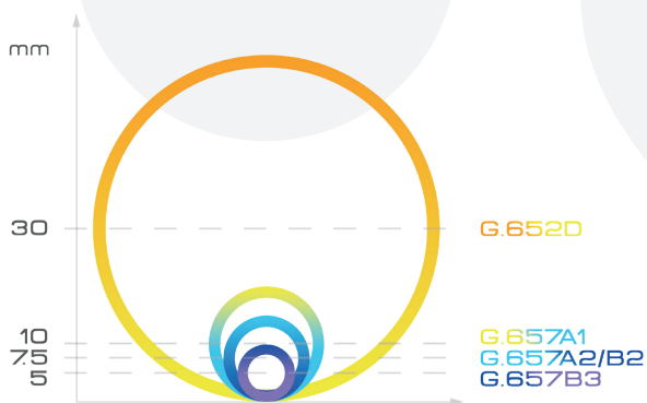
Minimal bending radius according to fibre type
