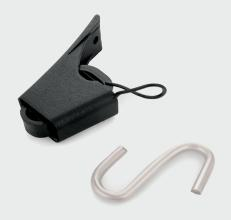
Anchoring cable clamp Sdünnger PA-FTTX-509 – an element used in the construction of aerial cable installations. It is responsible for maintaining adequate cable tension between spans. PA-FTTX-509 is dedicated for round and flat cables with a maximum diameter of up to 5.0mm. S-shaped metal hook (type 509) or detachable mounting eyelet (type 509-PL) enables easy installation of the cable clamp.
