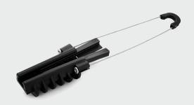
Anchoring cable clamp Sdünnger PA-37 v.2 - an element used in the construction of aerial cable installations. It is responsible for maintaining adequate cable tension between spans. The clamp can be placed on the outer sheath of the cable or on the supporting element (in the case of cables with an octagonal cross section, e.g. S-XOTKtc). Recommended for diameters from 3.0 to 7.0mm.
