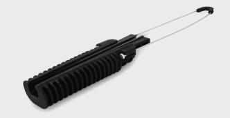
Anchoring cable clamp Sdünnger PA-200X-C – an element used in the construction of aerial cable installations. It is responsible for maintaining adequate cable tension between spans. The clamp can be placed on the outer sheath of the cable or on the supporting element (in the case of cables with an octagonal cross section, e.g. S-XOTKtc). Recommended for diameters from 8.0 to 12.0mm (PA-2000-C), 9.5 to 12.0mm (PA-2000-C v.2), 13.0 to 16.0mm (PA-2001-C), 16.0 to 20.0mm (PA-2002-C).
