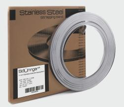
Steel banding tape Sdünnger F 197 (19x0.7mm, 32m), Stainless Steel 430 is used to create solid mounting straps. It is made of corrosion and weather resistant stainless steel 19mm wide and 0.7mm thick, packed in a 32m coil in a handy cardboard box.
