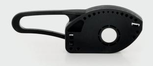
Anchoring cable clamp Sdünnger PA-FTTX-FISH-U – an element used in the construction of aerial cable installations. It is responsible for maintaining adequate cable tension between spans. PA-FTTX-FISH-U is dedicated for round and flat cables with a diameter of 2.5 to 4.0mm.
