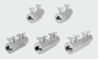
Cable screw connector Sdünnger - an element used to connect the conductors of wires. The universal hole allows the termination of single conductor and flexible conductors (cable). The use of two shear bolts ensures secure tightening of the conductor.
