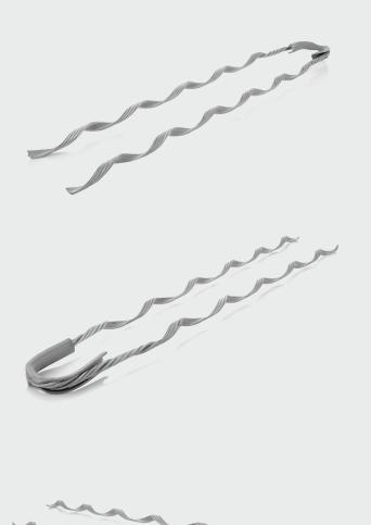
Anchoring cable clamp Sdünnger SPIRAL – an element used in securing of ADSS type cables. Used on wooden or concrete poles. It is mounted with the help of its central eyelet. An alternative to previous Sdünnger anchoring cable clamps. The clamp is made of an ASTM A475 standard steel wire, which is additionally hot dip galvanized.
