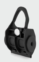
Suspension cable clamp Sdünnger D8 - an element used in the construction of aerial cable tracts for cable suspension. It is responsible for cable support between spans. The D8 clamp is suitable for selfsupporting, ADSS type round cables of a diameter between 8.0mm and 12.0mm.
