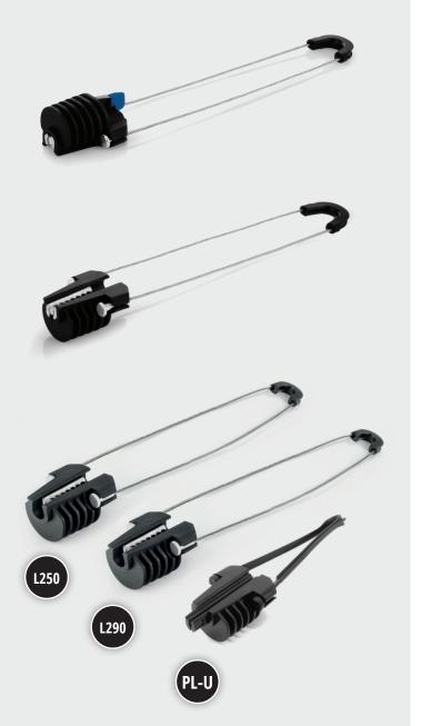
Anchoring cable clamp Sdünnger AC-05 - an element used in the construction of aerial cable installations. It is responsible for maintaining adequate cable tension between spans. The clamp can be placed on the outer sheath of the cable or on the supporting element (in the case of cables with an octagonal cross section, e.g. S-XOTKtc). Recommended for diameters from 3.0 to 6.0mm.
