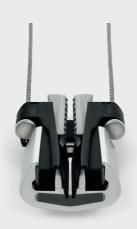
Anchoring cable clamp Sdünnger PAM-06- an element used in the construction of aerial cable installations. It is responsible for maintaining adequate cable tension between spans. The clamp can be placed on the outer sheath of the cable or on the supporting element (in the case of cables with an octagonal cross section, e.g. S-XOTKtc). Recommended for diameters up to 5.5mm.
