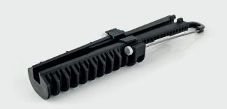
Anchoring cable clamp Sdünnger PA-2000-A - an element used in the construction of aerial cable installations. It is responsible for maintaining adequate cable tension between spans. The clamp can be placed on the outer sheath of the cable or on the supporting element (in the case of cables with an octagonal cross section, e.g. S-XOTKtc). Recommended for diameters from 9.5 to 12.0mm.
