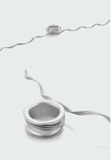
Suspension cable clamp Sdünnger SPIRAL – an element used in securing of ADSS type cables. Used on wooden or concrete poles. It is mounted with the help of its central eyelet. An alternative to previous Sdünnger anchoring cable clamps. The clamp is made of an ASTM A475 standard steel wire, which is additionally hot dip galvanized.
