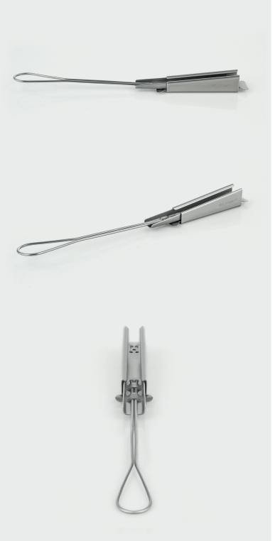
Anchoring cable clamp Sdünnger PA-FTTX-FLAT 2K – an element used in the construction of aerial cable installations. It is responsible for maintaining adequate cable tension between spans. PA-FTTX-FLAT 2K is designed for flat cables up to 11.0mm wide and 1.2 to 4.0mm thick.
