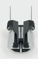
Anchoring cable clamp Sdünnger PAM-07- an element used in the construction of aerial cable installations. It is responsible for maintaining adequate cable tension between spans. The clamp can be placed on the outer sheath of the cable or on the supporting element (in the case of cables with an octagonal cross section, e.g. S-XOTKtc). Recommended for diameters up to 7.0mm.
