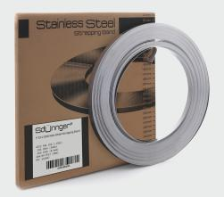
Steel banding tape Sdünnger F 104 (10x0.4mm, 50m), Stainless Steel 304 is used to create solid mounting straps. It is made of corrosion and weather resistant stainless steel 10mm wide and 0.4 mm thick, packed in a 50m coil in a handy cardboard box.
