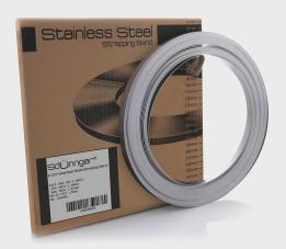
Steel banding tape Sdünnger F 107 (10x0.7mm, 30m), Stainless Steel 430 is used to create solid mounting straps. It is made of corrosion and weather resistant stainless steel 10mm wide and 0.7mm thick, packed in a 30m coil in a handy cardboard box.
