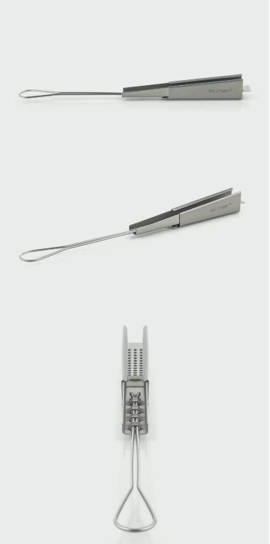
Anchoring cable clamp Sdünnger PA-FTTX-FLAT-BIG 4K – an element used in the construction of aerial cable installations. It is responsible for maintaining adequate cable tension between spans. PA-FTTX-FLAT-BIG 4K is designed for flat cables up to 14.0mm wide and 2.0 to 8.0mm thick, recommended for thickness from 2.0 to 7.0mm.
