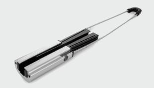
Anchoring cable clamp Sdünnger PA-170X-AL - an element used in the construction of aerial cable installations. It is responsible for maintaining adequate cable tension between spans. The clamp can be placed on the outer sheath of the cable or on the supporting element (in the case of cables with an octagonal cross section, e.g. S-XOTKtc). Recommended for diameters from 8.0 to 14.0mm (PA-1700-AL), 8.0 to 12.0mm (PA-1701-AL), 11.0 to 14.0mm (PA-1702-AL), 14.0 to 18.0mm (PA-1703-AL).
