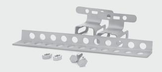
Transverse pole bracket Sdünnger 22/26/30 openings, with universal double sided base - an element used in the construction of multi-track aerial cable installations. It enables the mounting of anchoring and suspension cable clamps. Made of galvanized steel resistant to corrosion and weather conditions.
