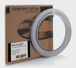
Steel banding tape Sdünnger F 137 (12.7x0.7mm, 30m), Stainless Steel 304 is used to create solid mounting straps. It is made of corrosion and weather resistant stainless steel 12.7mm wide and 0.7mm thick, packed in a 30m coil in a handy cardboard box.
