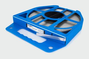
Steel banding tape Sdünnger F 107 (10x0.7mm, 50m), Stainless Steel 304 is used to create solid mounting straps. It is made of corrosion and weather resistant stainless steel 10mm wide and 0.7mm thick, packed in a 50m coil in a in a durable plastic packaging.
