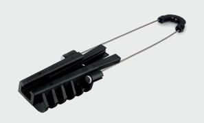
Anchoring cable clamp Sdünnger PA-69 v.2 - an element used in the construction of aerial cable installations. It is responsible for maintaining adequate cable tension between spans. The clamp can be placed on the outer sheath of the cable or on the supporting element (in the case of cables with an octagonal cross section, e.g. S-XOTKtc). Recommended for diameters from 6.0 to 9.0mm.
