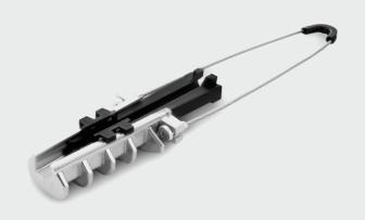
Anchoring cable clamp Sdünnger PA-1801-AL - an element used in the construction of aerial cable installations. It is responsible for maintaining adequate cable tension between spans. The clamp can be placed on the outer sheath of the cable or on the supporting element (in the case of cables with an octagonal cross section, e.g. S-XOTKtc). Recommended for diameters from 11.0 to 14.0mm.
