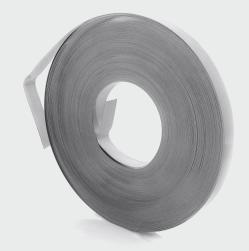
is used to create solid mounting straps. It is made of corrosion and weather resistant stainless steel 20mm wide and 0.4mm thick, packed in a 50m coil in a handy cardboard box.
