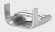
Buckle - clip for the Sdünnger A-200 (20mm) type L, Stainless Steel 304 banding tape. It is used to construct reliable fastening bands made of steel tape. Made of corrosion and weather resistant stainless steel, that is 1.50mm thick. A 20.4mm opening allows for use with F204 and F207 steel tape. Type L features a flat finish (no "teeth") - recommended in paring with thinner steel tapes.
