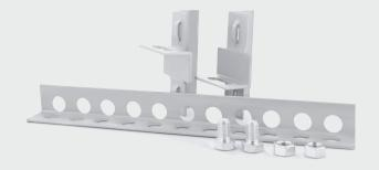
Transverse pole bracket Sdünnger 22/26/30 openings, with universal base - an element used in the construction of multi-track aerial cable installations. It enables the mounting of anchoring and suspension cable clamps. Made of galvanized steel resistant to corrosion and weather conditions.
