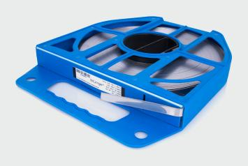
Steel banding tape Sdünnger F 197 (19x0.7mm, 50m), Stainless Steel 304 is used to create solid mounting straps. It is made of corrosion and weather resistant stainless steel 19mm wide and 0.7mm thick, packed in a 50m coil in a handy cardboard box.
