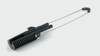
Anchoring cable clamp Sdünnger AC-10 - an element used in the construction of aerial cable installations. It is responsible for maintaining adequate cable tension between spans. The clamp can be placed on the outer sheath of the cable or on the supporting element (in the case of cables with an octagonal cross section, e.g. S-XOTKtc). Recommended for diameters from 5.0 to 8.0mm.
