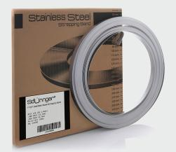
Steel banding tape Sdünnger F 137 (12.7x0.7mm, 30m), Stainless Steel 430 is used to create solid mounting straps. It is made of corrosion and weather resistant stainless steel 12.7mm wide and 0.7mm thick, packed in a 30m coil in a handy cardboard box.
