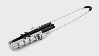
Anchoring cable clamp Sdünnger PA-1001-AL - an element used in the construction of aerial cable installations. It is responsible for maintaining adequate cable tension between spans. The clamp can be placed on the outer sheath of the cable or on the supporting element (in the case of cables with an octagonal cross section, e.g. S-XOTKtc). Recommended for diameters from 7.0 to 11.0mm.
