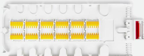
Tycon C1 - splice tray designed for organizing optical fibers in fiber optic closures and enclosures. The tray can accommodate up to 72 splices. Trays can be stacked, facilitating the installation process. Recommended splice protector length: up to 45 mm.
