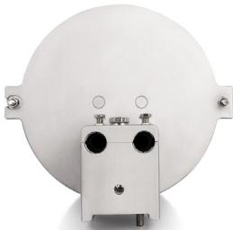
Tycon OPGW are dome closures used for overhead power line lightning protection conductors containing optical fibers (OPGW), as well as for ADSS cables. They have an IP65 protection rating. The body is made entirely of aluminum and is designed for straightforward and efficient installation. The organization of fiber optic strands inside the closure is facilitated by integrated fiber optic trays. All metal components of the closures are made from corrosion-resistant materials.
