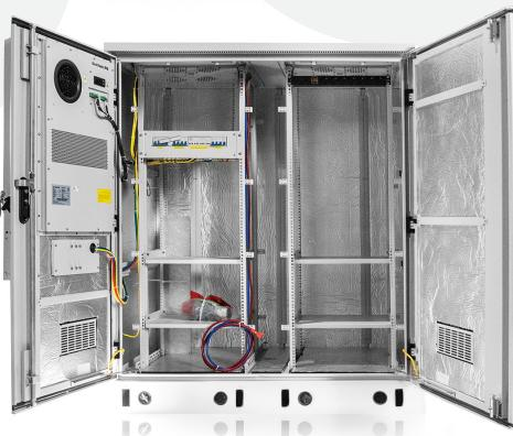
A freestanding cabinet with a height of 42U, designed for outdoor use. Constructed from 1.5 mm thick 201 stainless steel, providing high strength and resistance to harsh environmental conditions. The cabinet features 20 mm polyurethane insulation and automatic temperature control - if the internal temperature exceeds 35 °C, the air conditioner is activated automatically.
