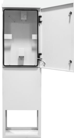
The Tycon FTTH pedestal cabinet is designed for outdoor installation by embedding it in the ground to a depth of approximately 60 cm, ensuring stable placement. The design allows convenient mounting of a fiber optic closure, and the thoughtfully organized interior facilitates installation and orderly management of fiber optic cables.
