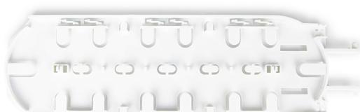
Tycon B2 - splice tray designed for organizing optical fibers in fiber optic closures and enclosures. The tray can accommodate up to 24 splices. Trays can be stacked, facilitating the installation process. Recommended splice protector length: up to 45 mm.
