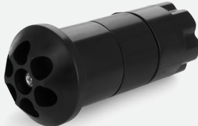
Mechanical sealing for the round port of the Tycon 500 C6 closure for 6 cables up to 8.3 mm - allows replacing the thermal sealing of the round port with a mechanical seal. It features 6 inlets with a diameter of 8.3 mm.
