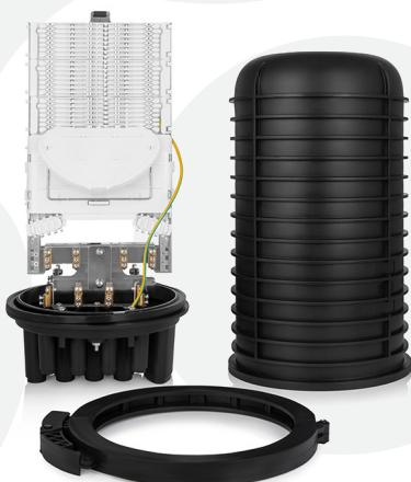
The closure is equipped with fully hermetic, heat-shrinkable inlet/outlet ports. It is used to protect fiber optic cable splices and for branching applications. The housing is made of high-quality plastic resistant to UV radiation, low (-40°C) and high (+60°C) temperatures, as well as chemical substances, making it suitable for aerial, duct, and direct-buried installations. It has an IP68 protection rating.
