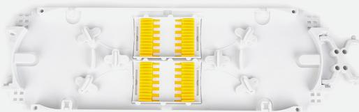
Tycon A1 - splice tray designed for organizing optical fibers in fiber optic closures and enclosures. The tray can accommodate up to 24 splices. Trays can be stacked, facilitating the installation process. Recommended splice protector length: up to 45 mm.
