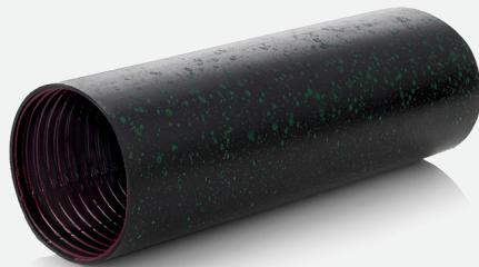
The Tycon heat-shrink sleeve is a heat-shrinkable cover with adhesive designed for the protection, sealing, and mechanical reinforcement of fiber optic cables at their entry points into closures and telecommunications enclosures. When heated, it shrinks to fit tightly around the cable and the edges of the opening, providing effective protection against moisture, dust, and other external factors.
