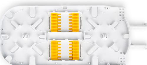
Tycon E1 - splice tray designed for organizing optical fibers in fiber optic closures and enclosures. The tray can accommodate up to 24 splices. Trays can be stacked, facilitating the installation process. Recommended splice protector length: up to 45 mm.
