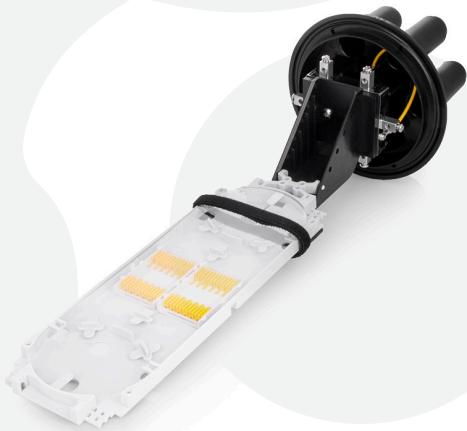
The closure is equipped with fully hermetic, heat-shrinkable inlet/outlet ports. It is used to protect fiber optic cable splices and for branching applications. Fiber management inside the closure is facilitated by fiber optic splice trays, which can be purchased separately. The housing is made of high-quality plastic resistant to UV radiation, low (-40°C) and high (+60°C) temperatures, as well as chemical substances, making it suitable for aerial, duct, and direct-buried installations.
