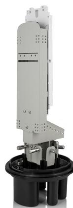
The closure is equipped with fully hermetic, heat-shrinkable inlet/outlet ports. It is used to protect fiber optic cable splices and for branching applications. The housing is made of high-quality plastic resistant to UV radiation, low (-40°C) and high (+60°C) temperatures, as well as chemical substances, making it suitable for aerial, duct, and direct-buried installations. It has an IP68 protection rating.
