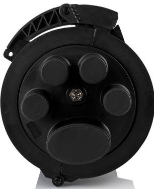
The closure is equipped with fully hermetic, heat-shrinkable inlet/outlet ports. It is used to protect fiber optic cable splices and for branching applications. Fiber management inside the closure is facilitated by fiber optic splice trays, which can be purchased separately.
