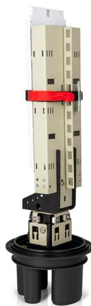
The closure is equipped with fully hermetic, heat-shrinkable inlet/outlet ports. It is used to protect fiber optic cable splices and for branching applications. The housing is made of high-quality plastic resistant to UV radiation, low (-40°C) and high (+60°C) temperatures, as well as chemical substances, making it suitable for aerial, duct, and direct-buried installations. It has an IP68 protection rating.
