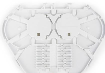
Tycon D1-1S-08F SPLITTER - splice tray designed for organizing optical fibers in fiber optic closures and enclosures. The tray can accommodate up to 4 splices and the installation of a PLC splitter. Trays can be stacked, facilitating the installation process.
