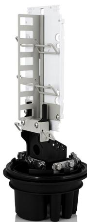
The closure is equipped with fully hermetic, heat-shrinkable inlet/outlet ports. It was designed based on the construction of the Tycon 400 fiber optic closure A8-T-000 096J-04xS A8-000. It is extended with an integrated patch panel, allowing the installation of up to 24 fiber optic adapters in SC Simplex format (or LC Duplex format). By using the patch panel with SC Simplex adapters, installation time and costs can be significantly reduced.
