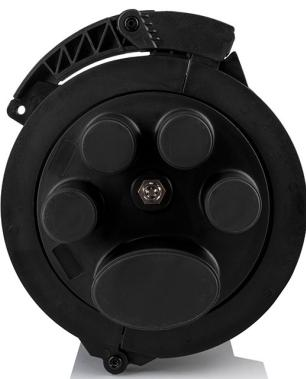
The closure is equipped with fully hermetic, heat-shrinkable inlet/outlet ports. It is used to protect fiber optic cable splices and for branching applications. Fiber management inside the closure is facilitated by fiber optic splice trays, which can be purchased separately. The basket allows the installation of two splitters (1x8 STEEL and 1x16 STEEL).
