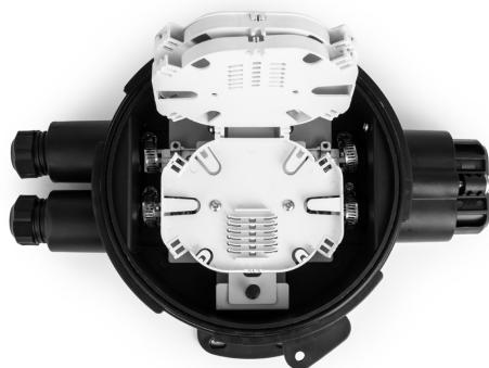
Horizontal closure, equipped with 4 inlet/outlet ports. This type of closure is used to protect fiber optic cable splices and branching applications. The closure is designed for simple and efficient installation. The organization of fiber optic strands in the closure is facilitated by three fiber optic trays, each accommodating 7 splices (can be arranged in double layers).
