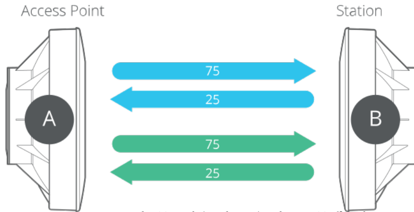
Figure 10 – Example PTP Link (Single Hop) with 75/25 Traffic Split
